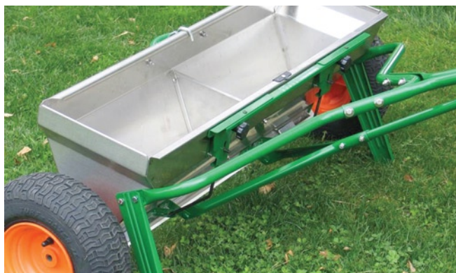
Figure 10.2. A typical 3-foot-wide drop (gravity-fed) spreader.
