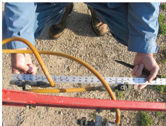
Figure 10.16. Nozzles should be equally spaced on the boom according to manufacturer recommendations. By measuring the spacing, you can then calculate the test course length in order to calibrate the sprayer according to the ounce calibration method.
