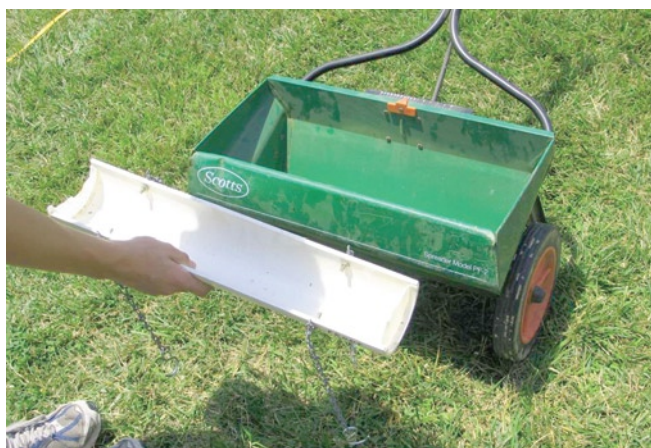
Figure 10.5. A homemade catch pan made from a piece of PVC pipe.
