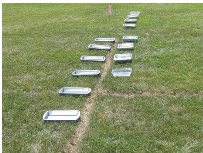
Figure 10.9. Fertilizer catch pans are being placed at regular intervals in order to determine the fertilizer's effective distribution width.
