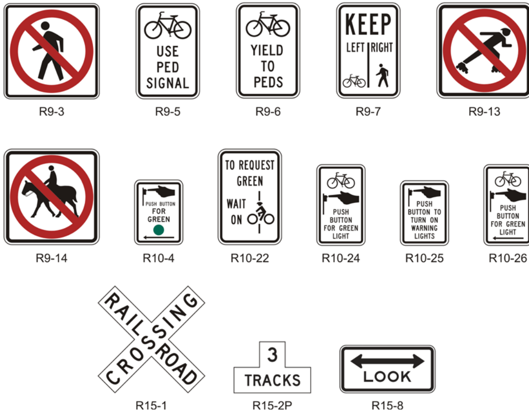
Figure 9B-2. Regulatory Signs and Plaques for Bicycle Facilities (Sheet 2 of 2) (Delaware Revision)
