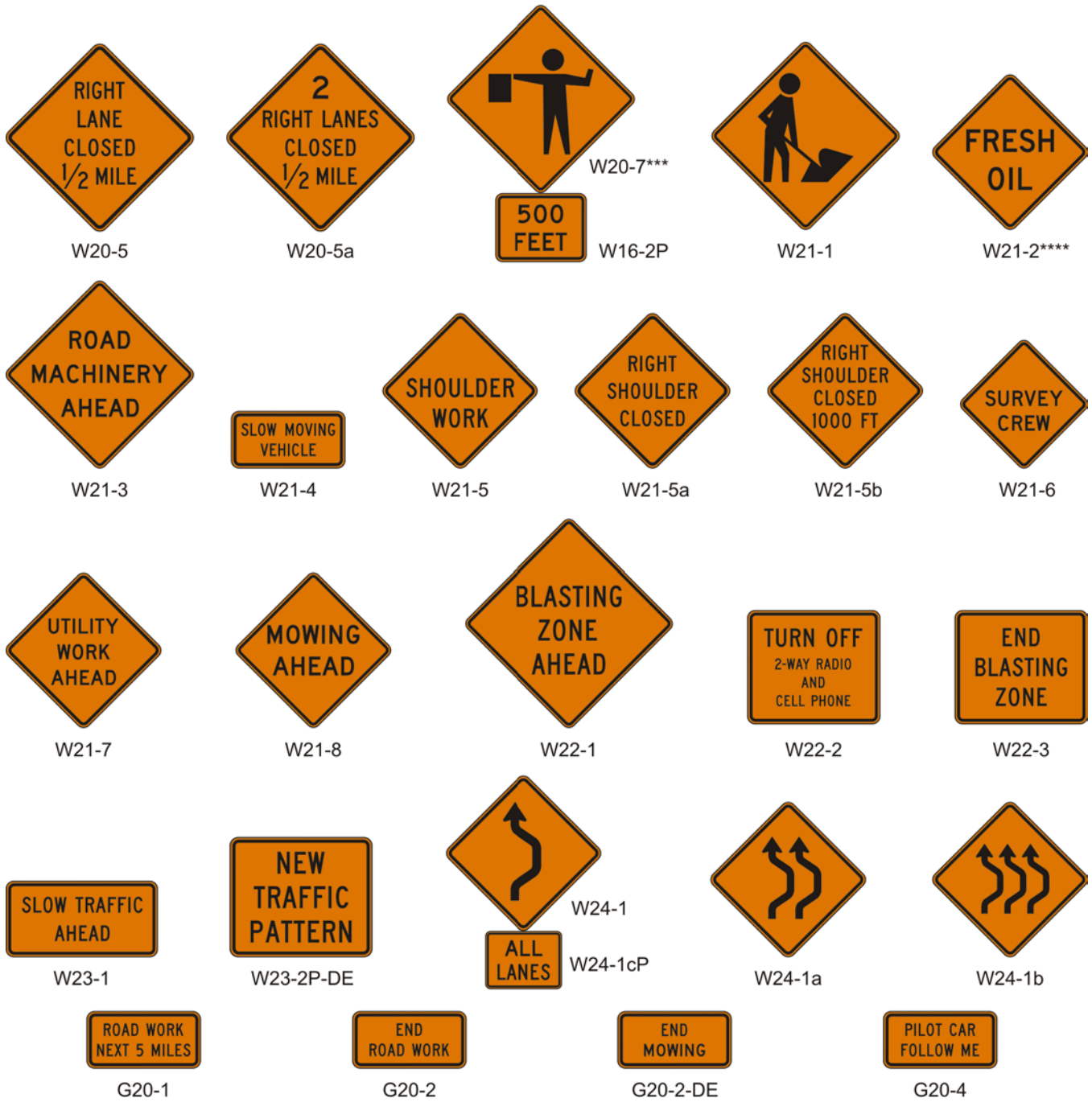
Figure 6F-4. Warning Signs and Plaques in Temporary Traffic Control Zones (Sheet 3 of 3) (Delaware Revision)
