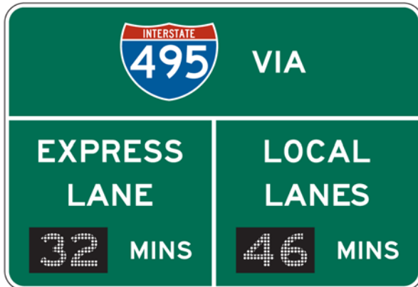
Figure 2G-20. Example of a Comparative Travel Time Information Sign for Preferential or Managed Lanes
