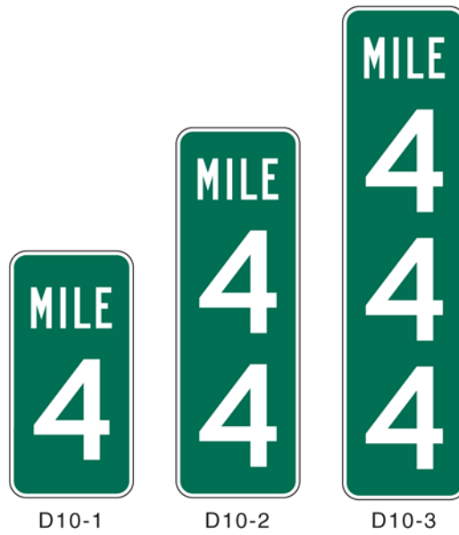
Figure 2H-2. Reference Location Signs
