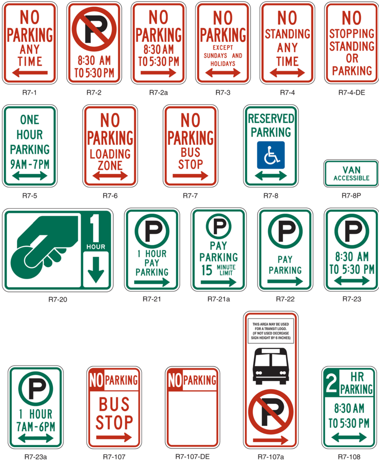
Figure 2B-24. Parking and Standing Signs and Plaques (R7 Series) (Sheet 1 of 2) (Delaware Revision)
