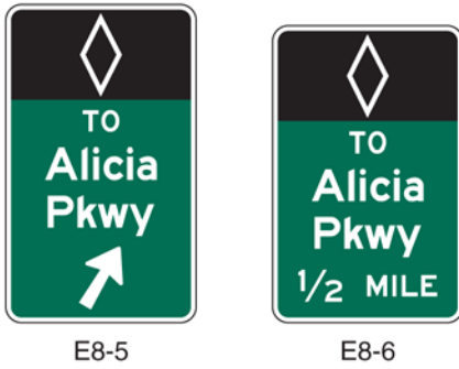
Figure 2G-11. Examples of Barrier-Mounted Guide Signs for an Intermediate Egress from Preferential Lanes
