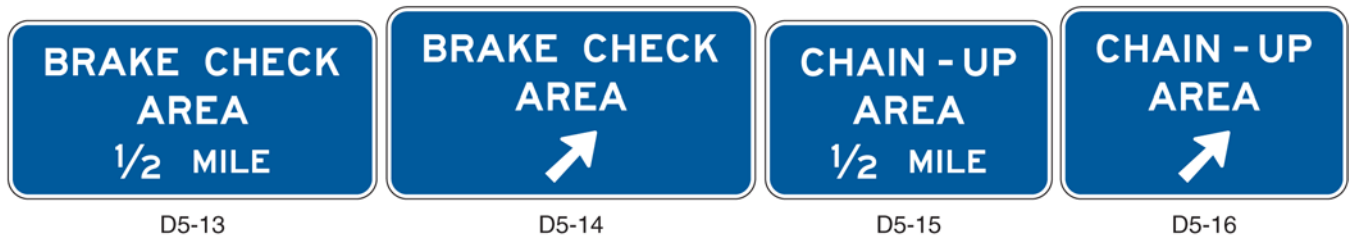
Figure 2I-6. Brake Check Area and Chain-Up Area Signs
