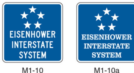
Figure 2E-18. Eisenhower Interstate System Signs
