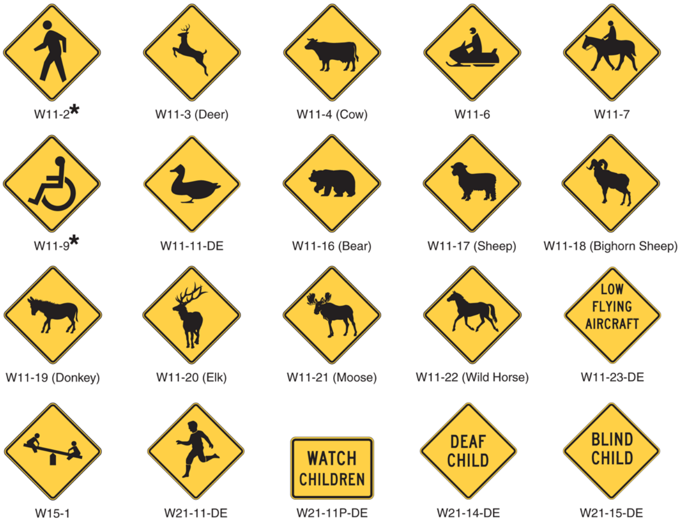
Figure 2C-11. Non-Vehicular Warning Signs (Delaware Revision)
