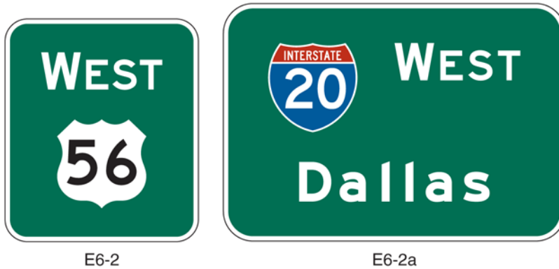
Figure 2E-2. Pull-Through Signs
