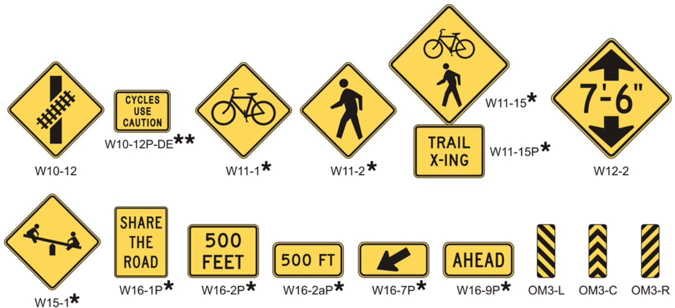
Figure 9B-3. Warning Signs and Plaques and Object Markers for Bicycle Facilities (Sheet 2 of 2) (Delaware Revision)
