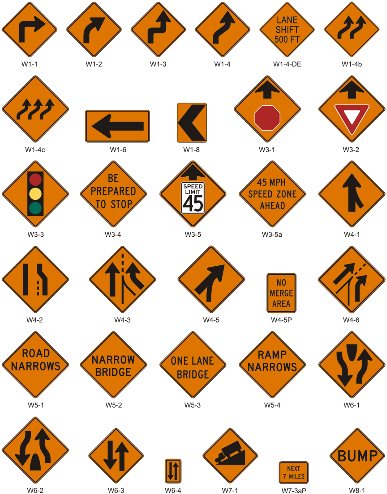
Figure 6F-4. Warning Signs and Plaques in Temporary Traffic Control Zones (Sheet 1 of 3) (Delaware Revision)
