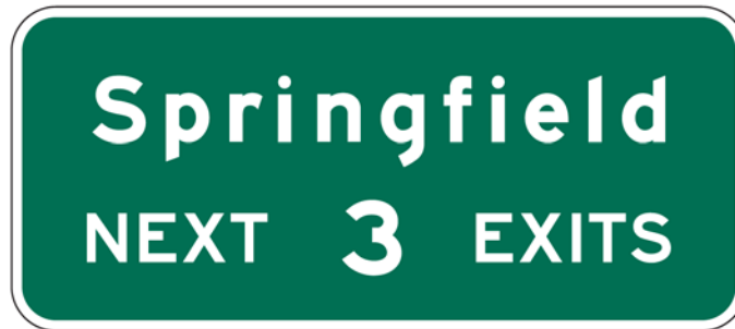
Figure 2E-33. NEXT EXITS Sign
