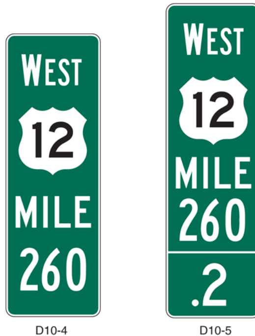
Figure 2H-4. Enhanced Reference Location Signs
