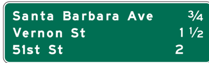
Figure 2E-31. Interchange Sequence Sign
