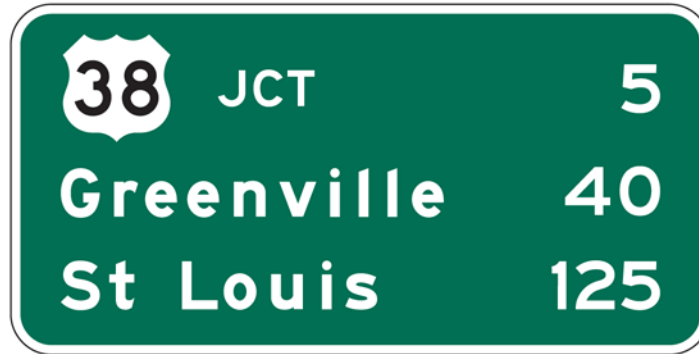
Figure 2E-29. Post-Interchange Distance Sign
