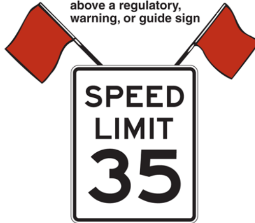
Figure 2A-1. Examples of Enhanced Conspicuity for Signs
