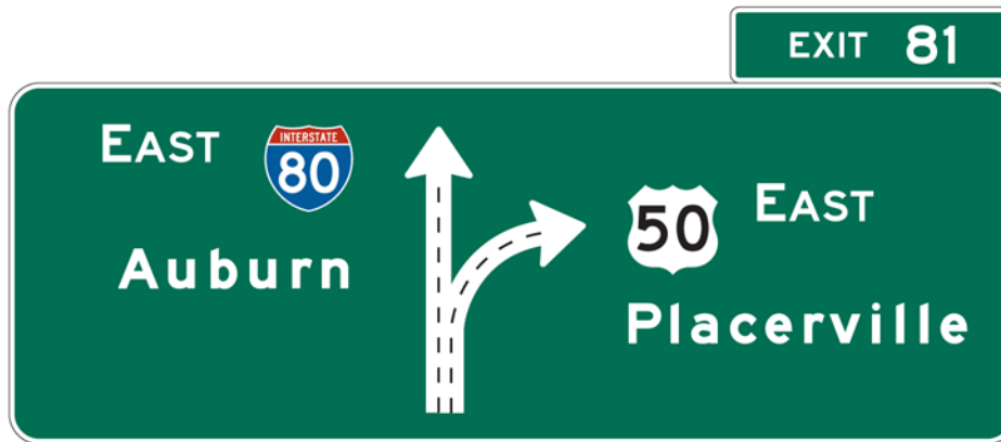
Figure 2E-7. Diagrammatic Guide Sign for a Multi-Lane Exit with an Option Lane
