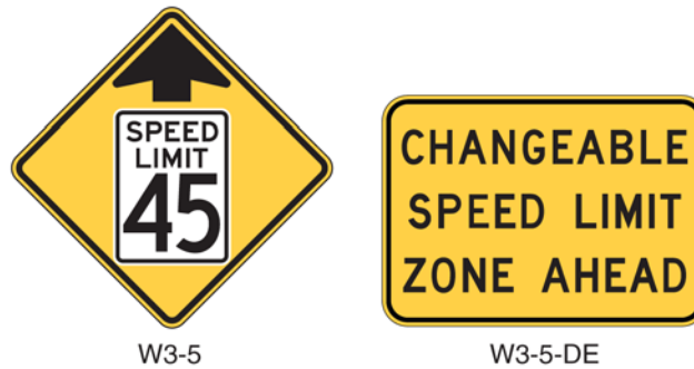
Figure 2C-7. Reduced Speed Limit Ahead Signs (Delaware Revision)
